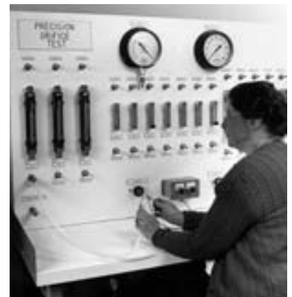
All production orifices are flow tested and must meet exacting flow standards. A special test bench has been constructed for this purpose.
