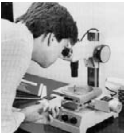
Orifice diameter dimensions are checked using a precision measuring microscope. Accuracy is better than .0001".
