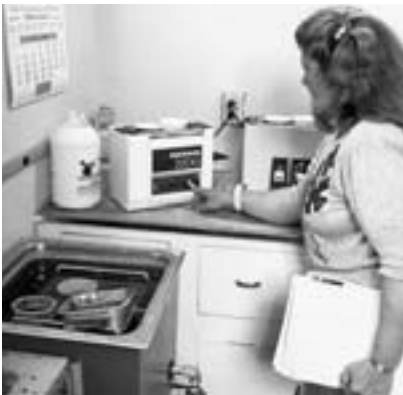
Ultrasonic cleaners are used to remove contamination from the interior of orifice assemblies. Small particles can cause major changes in orifice flow rates.
