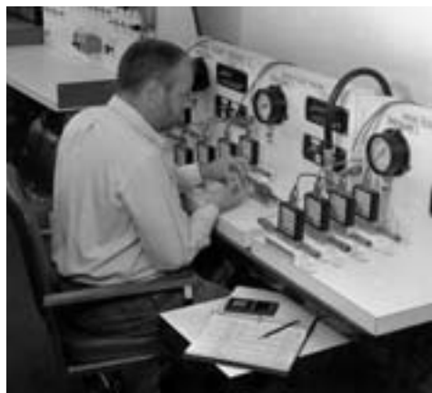
Mass flowmeters are used for NIST traceable calibration of orifice flow.
