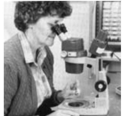
All production orifices are examined by experienced inspectors using a microscope to detect contaminants and to assure orifice quality.
